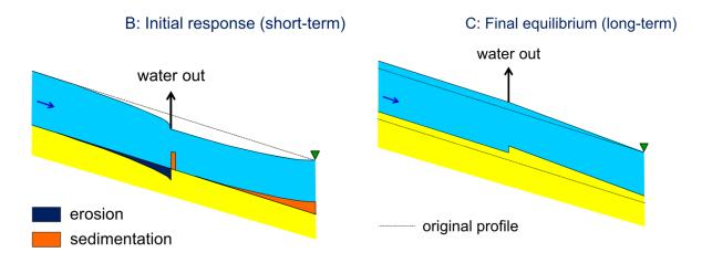
Figure 2.3 Physics-based diagram of elementary short-term and long-term hydromorphological responses to water abstraction.
